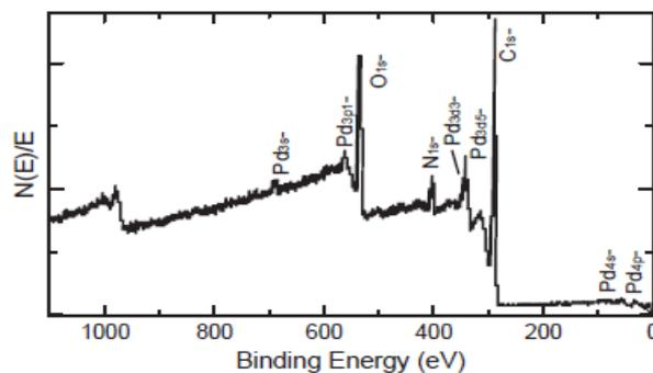
Fig.4 XPS survey spectra of Kevlar® fabric (T732) impregnation with  $\text{Pd}(\text{hfa})_2$  (1.0 wt%) at 150 °C and 15 MPa for 15 min.
