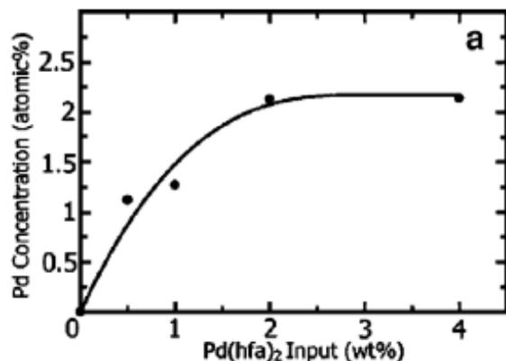
Fig.6 Effect of the amount of Pd(hfa)<sub>2</sub> on the Pd concentration. The Pd(hfa)<sub>2</sub> was impregnated into the Kevlar® fabric (T732) using scCO<sub>2</sub> at 150 °C and 15 MPa.
