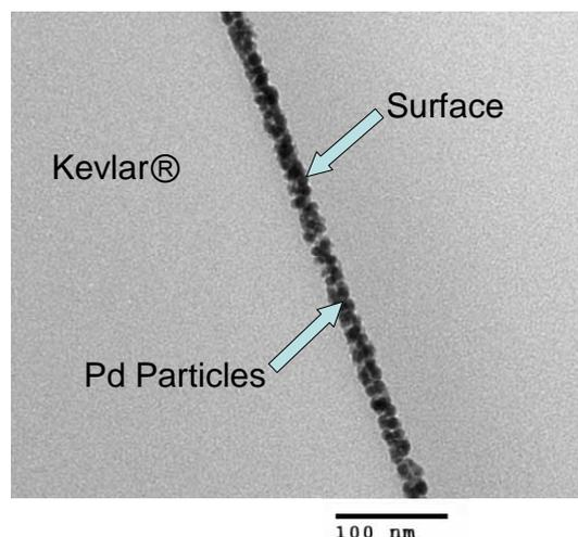
Fig.10 TEM image for cross-section of Pd-impregnated Kevlar fiber. Pd particles are distributed in the fiber.
