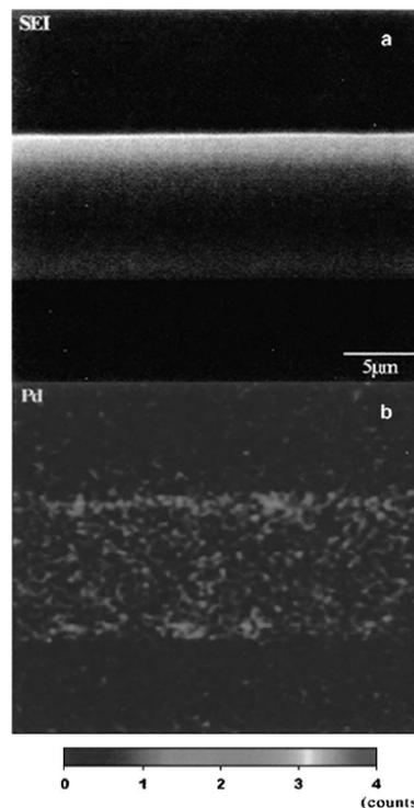
Fig.5 Surface image analysis of Kevlar®-29 fiber impregnation with  $\text{Pd}(\text{hfa})_2$  (1.0 wt.%) at 10 MPa and 150 °C for 15 min. (a) SEI (Secondary Electron Imaging) image, (b) EPMA image.
