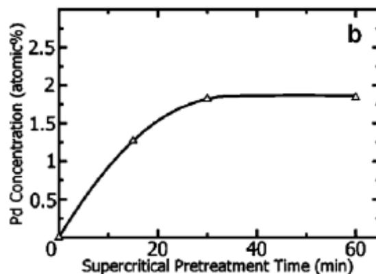
Fig.9 Effect of the supercritical pretreatment time on the Pd concentration. The Pd(hfa)<sub>2</sub> was impregnated into the Kevlar® fabric (T732) using scCO<sub>2</sub> at 150 °C and 15 MPa.
