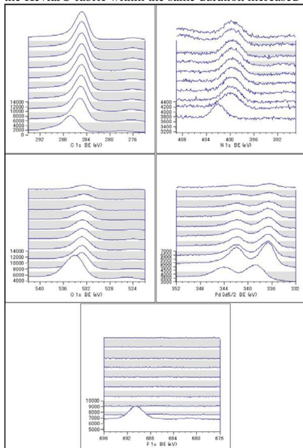
Fig.7 XPS depth profile for aramid fiber surface after SCF-Palladium (II)-hexafluoroacetylacetonate impregnation for 3 h and thermal treatment for 1 h showing the differences between the chemical shifts of C 1s, N 1s, O 1s, Pd 3d<sub>5/2</sub>, Pd 3d<sub>3/2</sub>, and F 1s atoms in the surface and deeper regions and the high detection of Pd peaks in depth
