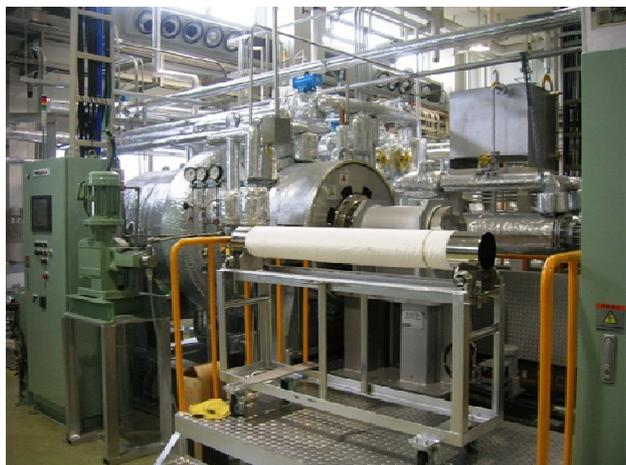
Fig.11 Practical supercritical fluid plant having 350 liters treating bath for fiber and textile treatments.
