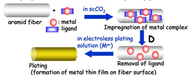
Fig.2 Process of electroless plating of aramid Fibers using  $scCO_2$ .
