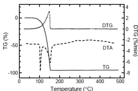
Fig.3 Combined thermogravimetric(TG), differential thermo-gravimetric (DTG), and differential thermal analytic (DTA) curves of  $\text{Pd}(\text{hfa})_2$  in a dynamic argon atmosphere.
