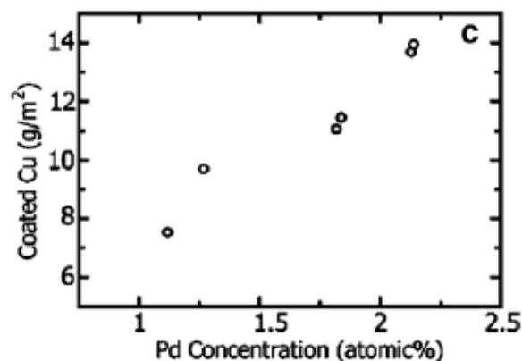
Fig.8 Effect of the Pd concentration on the amount of Cu coating after electroless copper plating under magnet stirring for 5 min at 42 °C. The Pd(hfa)<sub>2</sub> was impregnated into the Kevlar® fabric (T732) using scCO<sub>2</sub> at 150 °C and 15 MPa.
